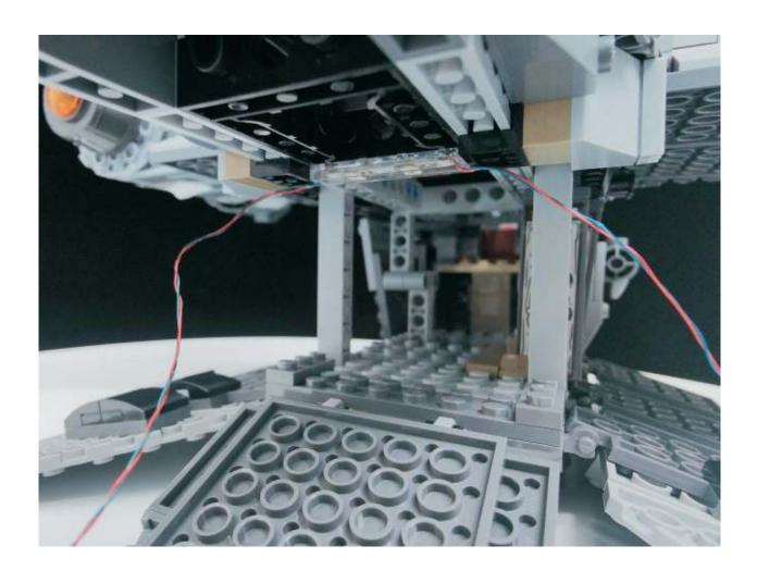
Pass the wire through the blocks and install the second lamp set as follows
